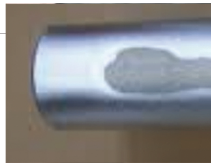
Diagram 5 showing Zinc coating drips
