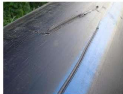
Diagram 3 showing a longitudinal scratch
